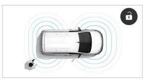
"zoning" function For locking or unlocking either the front doors or the loading area.
