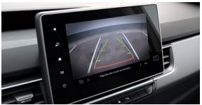
**rear-view camera.** It provides a rearward view on the easy link screen or the interior rear-view mirror when you engage reverse gear. Superimposed outlines make your manoeuvres easier and cafer
