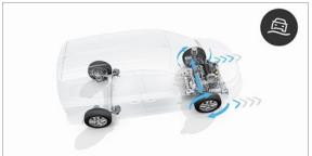
**Grip Xtend.** It allows you to drive in all weathers on different types of terrain (mud, leaves, rough roads, etc.). The system combines electronic stability control (ESC) and all-weather tyres to bring you enhanced traction, available at speeds of up to 50km/h.
