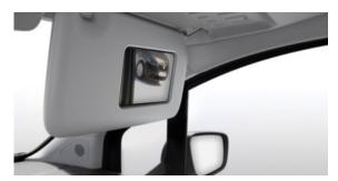
wide view mirror. Located in the passenger sun visor, it improves your vision and helps to minimise the effect of blind spots at Y-junctions. Available as standard on Advance models.
