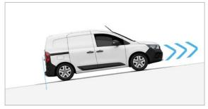
hill start assist. Combined with ESC, hill start assist maintains brake pressure automatically for 2 seconds to give you time to lift your foot from the brake pedal and press the accelerator. The system activates when the slope exceeds 3%. Available as standard on all models.
